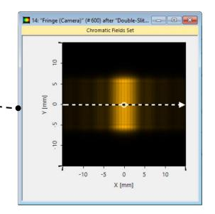
The partial coherence of the physical extended source which leads to a blurring of the interference fringes is here modeled with the set of self-correlated but mutually incoherent point sources presented in the previous slide. The interference patterns of each of the point sources do not coincide, causing the characteristic loss of contrast.
