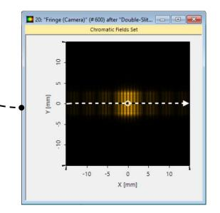
By increasing the propagation distance in front of the double slit to 1500mm, we demonstrate the predictions of the van Cittert-Zernike theorem, in that the light generated from two incoherent sources will appear coherent from far away. This is evidenced by the increase in contrast that occurs for a larger distance in front of the double slit.
