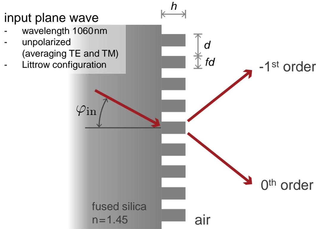
The diffraction efficiency of the -1<sup>st</sup> order, with unpolarized incidence, is to be calculated.
