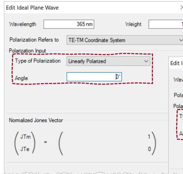
We set the incident plane wave in the TE-TM coordinate system, with linear polarization angles  $0^\circ$  and  $90^\circ$ , here for normal incidence, exactly along x- and y-direction.
