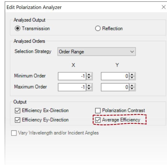
The polarization analyzer does the job of averaging the diffraction efficiencies for selected orders, with  $E_x$  and  $E_y$  polarizations as the input.
