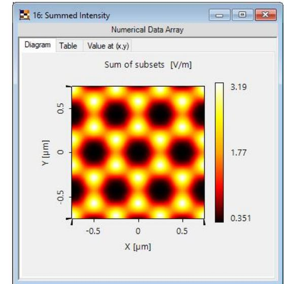
The resulting Talbot images are independent of the choice of the two orthogonal input polarization states.
