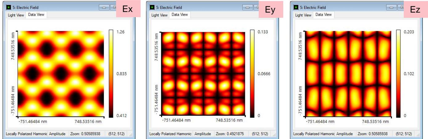
transmitted field components from y-polarized input
