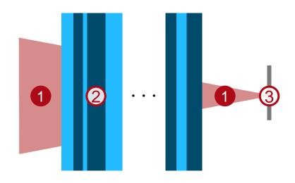
As the propagation to the focus must include diffractive effects in order to achieve an accurate result, the **Fourier Domain Techniques** are chosen as a good compromise between speed and accuracy for the simulation.
