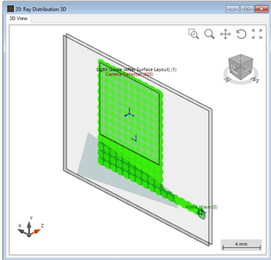
*Rays in System* view with  $32^\circ \times 18^\circ$  scanning source input (9 modes, differently colored):
