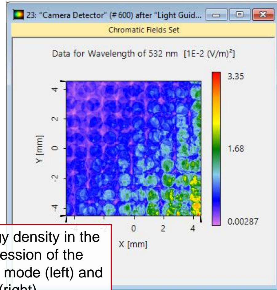
The distribution of the energy density in the eye box provides an impression of the lateral uniformity for a single mode (left) and for several modes (right).
