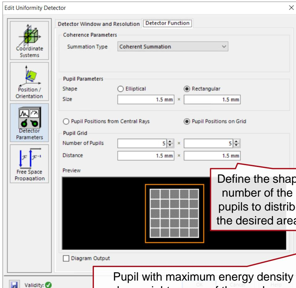
Pupil with maximum energy density is at the lower right corner of the eye box, while the minimum is at the top left corner.
