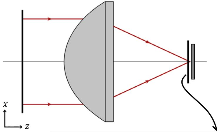
Fully vectorial simulation of light propagation through high-NA lens takes only 4 seconds!
