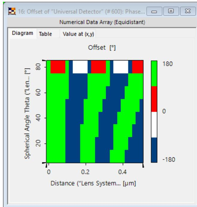
At or near the red-green boundaries, the phase offset is expected to be  $+90^\circ$ , while at or near the blue-white boundaries, it should be  $-90^\circ$ .
