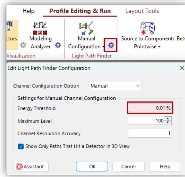
Based on the convergence, the default *Energy Threshold* of 0.01% appears sufficient to achieve  $\sim 0.5^\circ$  accuracy for the current setup and will therefore be used moving forward.
