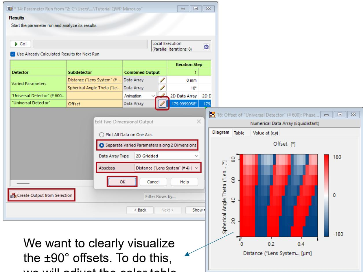
We want to clearly visualize the  $\pm 90^\circ$  offsets. To do this, we will adjust the color table so that the plot changes color precisely at  $\pm 90^\circ$ .
