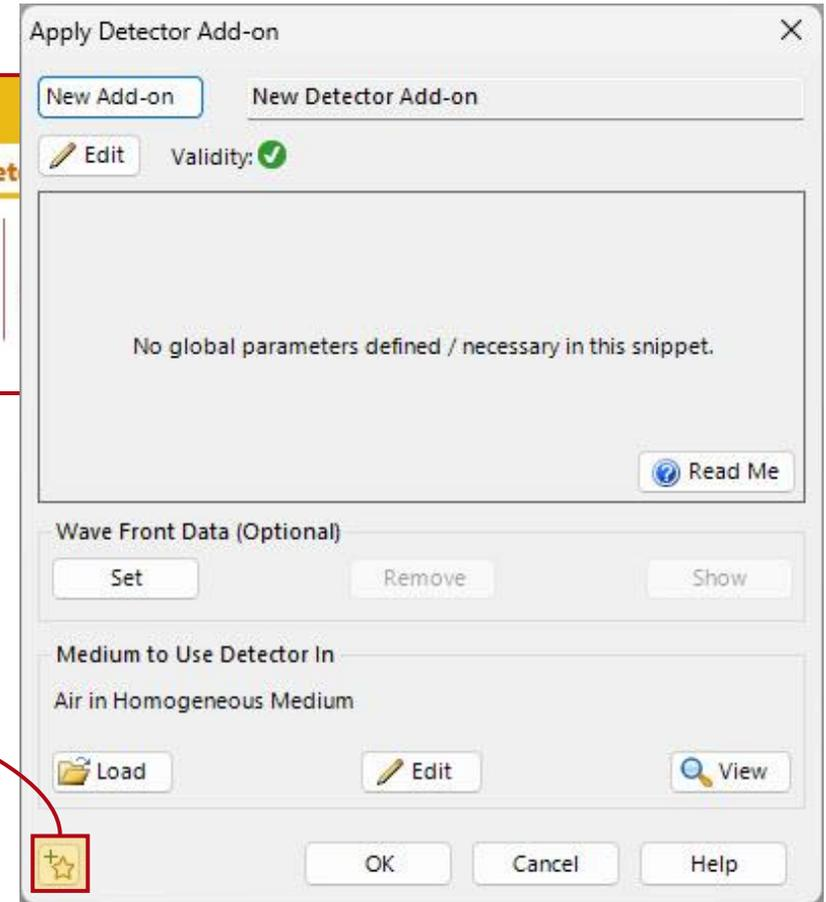
Under *Detectors/Apply Detector Add-on* the user can apply any predefined or customized *Detector Add-ons* to a *Data Array* to further post-process the results.
