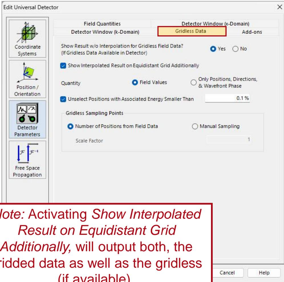
*Note: Activating Show Interpolated Result on Equidistant Grid Additionally, will output both, the gridded data as well as the gridless (if available).*
