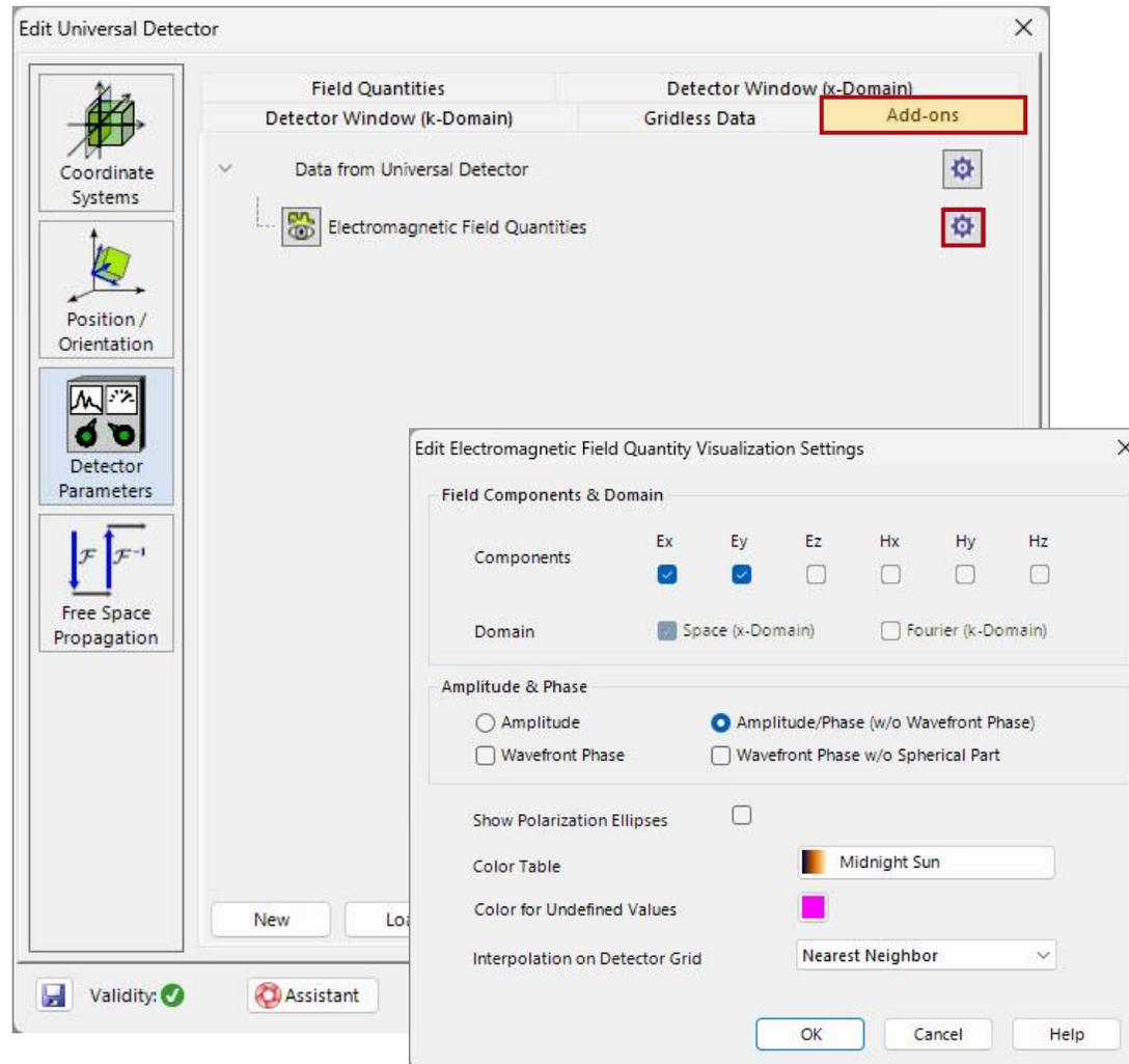
*Add-ons* are versatile tools that allow for an additional calculation of any values based on the impinging field data (either single physical values or 2D arrays). They are organized in tree, for the case the one add-on requires the result of another.
