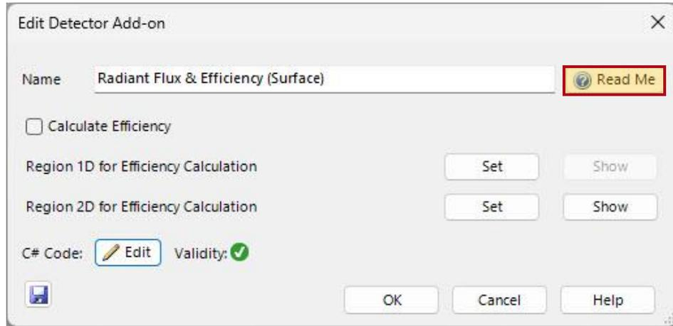
Every *Add-on* from the official database comes with a read-me document, explaining its functionality and stating the input and output parameters.
