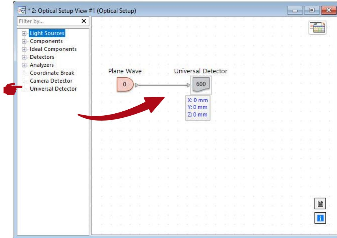
The *Universal Detector* can be found in the tree of components in *Light Path Editor*, directly. To add it to your system, simply drag & drop it to the desired position.
