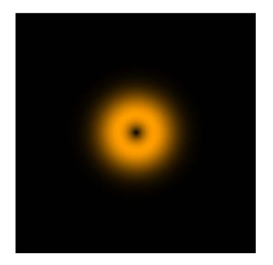
By means of the example, it is intended to illustrating the access on field values in a Programmable Detector via source code. The programmable detector calculates the sum of all squared amplitudes on the optical axis including all field components. As an example, the detector is applied on a donut mode, which is modeled as the combination of a  $HG_{01}$  and a  $HG_{10}$  Hermite Gaussian modes.
