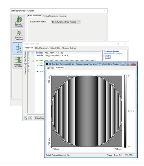
Providing maximum versatility for your optical simulations is one of our most fundamental objectives. In this tutorial we explain how to work with the Programmable Function, which can also be thought of as an idealised component acting in a single plane: the workflow entails defining a position-dependent, complex-valued function on the x, y plane, which is then multiplied onto the incoming field. We use the example of an ideal cylindrical lens to go through the whole process in detail.
