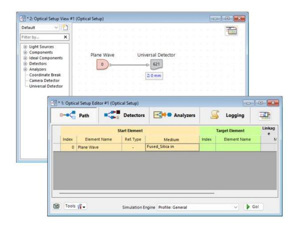
The main purpose of VirtualLab Fusion is to bring the experiments and research from the real world into a virtual one, with the Optical Setup serving as a kind of digital twin to a real-life laboratory. Here, the user can configure sources, components and detectors, control the positions and parameters of all components as well as define the materials that fill the space between them. This use case provides a general introduction to the concept.
