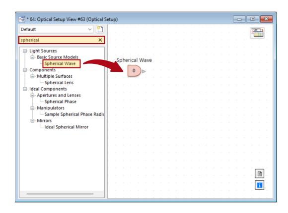
Once an element has been dropped on the right side, it also will automatically appear as an entry in the *Optical Setup Editor*.
