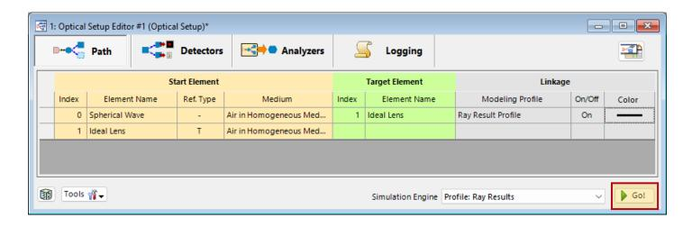
To actually perform the simulation, simply click on the *Go!* button either in the *Optical Setup Editor* or in the *Profile Editing & Run* menu tab. VirtualLab Fusion will then automatically start the simulation using the active *Simulation Profile*. For more information on how to configure your simulation, take a look at the following documentation:
