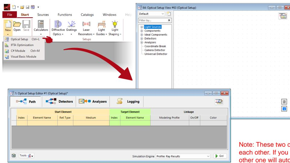
Clicking on New and Optical Setup in the Start ribbon will automatically generate two empty documents: The Optical Setup View, where the overall structure and positioning of your system is visualized, and the Optical Setup Editor, that can be used to configure other aspects of the system, like changing the material that fills the space between two elements, for instance.
