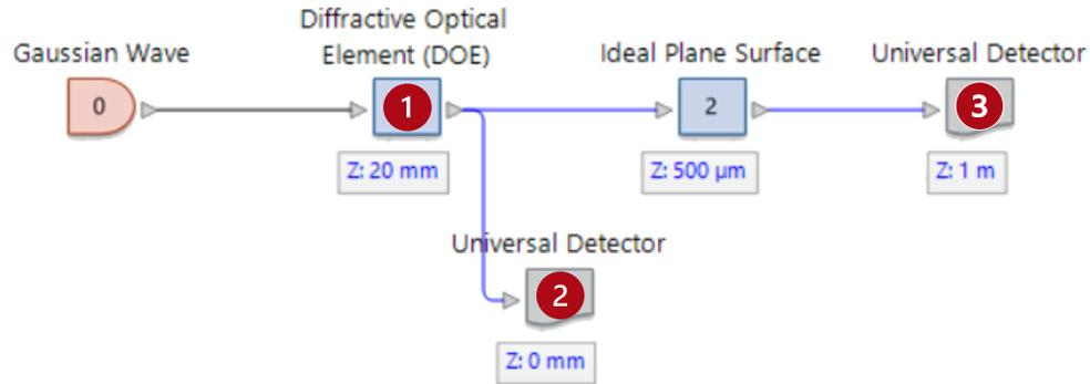
We constructed a diffractive beam splitter using the imported DOE. The phase profile immediately after the DOE mirrors the height profile loaded from the DOE. From the far field picture, we can observe that the DOE functions as a  $5 \times 5$  beam splitter. This can be further optimized by adjusting parameters such as the refractive index.
