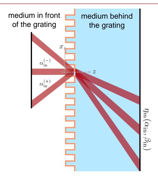
As a result, the detector calculates the mean efficiency and the uniformity contrast according to the efficiencies as a function of the incident directions of a set of plane waves for a specific diffraction order m.
