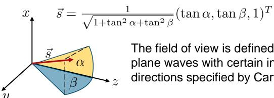
The field of view is defined as a set of plane waves with certain incident directions specified by Cartesian angles.
