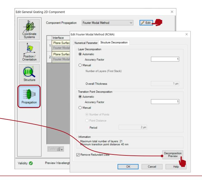
If the numbers of layers and transition points are increased (e.g. by a factor of 2), the discretization becomes less rough. (because a medium is sampled both values have to be increased)
