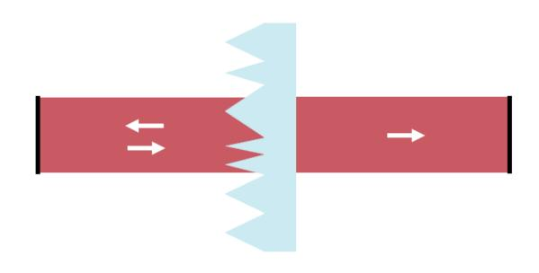
Minimizing reflection on optical surfaces is of great importance for various optical applications. An intriguing method to mitigate surface reflection involves the employment of nano- and micro-structures designed to counteract reflection, drawing inspiration from natural phenomena such as moth-eye structures. In this use case, we intend to investigate the overall reflection of such a structure by applying tolerance analysis within the framework of VirtualLab Fusion.
