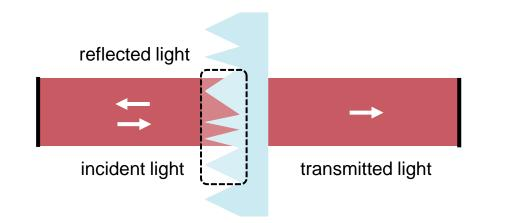
The overall reflectance is evaluated by varying the number of cones, height of cones and base diameter of the cones separately. Such a variation of parameters can be achieved by a *Parameter Run.*
