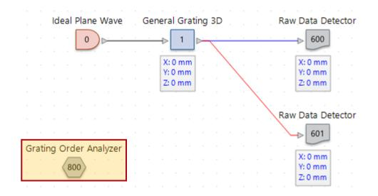
The *Grating Order Analyzer* can be used to investigate the efficiency of the diffraction orders of a given grating. Find more information under:
