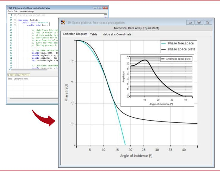
The space plate can reduce the required propagation distance by imitating the phase response of a free-space propagation step for a desired range of incident angles. A C# module was used to compute and visualize this phenomenon in a format similar to the reference. In comparison to the figure below, the result is reproduced in VirtualLab Fusion.
