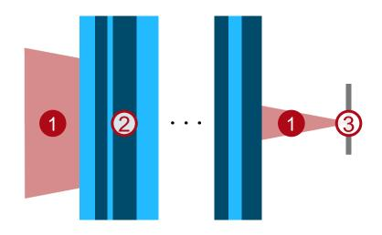
As the propagation to the focus must include diffractive effects in order to achieve an accurate result, the **Fourier Domain Techniques** are chosen as a good compromise between speed and accuracy for the simulation.
