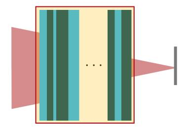
We use the *Stratified Media Component* to model the multi layer structure of the space plate, since it provides a fast and rigorous solution for lateral invariant layer stacks.
