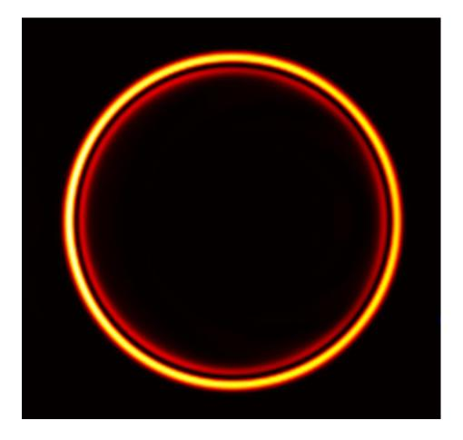
Conical refraction is a well-know phenomenon occurring in biaxial crystals, whereby an input Gaussian beam is transformed into a light ring whose intensity distribution is related to the incoming polarization. Several applications have been developed based on this phenomenon, polarization metrology among them. In this use case, we demonstrate the design of a polarimeter with two biaxial crystals, one in each arm of the setup, utilizing the fast physical-optics software VirtualLab Fusion.
