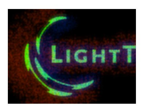
Micro-optical elements, like gratings, prisms and mirrors can be arranged to deflect light into expected direction and so to generate customized patterns. Such cells arrays are often used behind LED sources, and the design of cells arrays requires proper consideration on colors and coherence. In this example, cells arrays consisting of gratings, prisms and mirrors are designed to generate a LightTrans logo.
