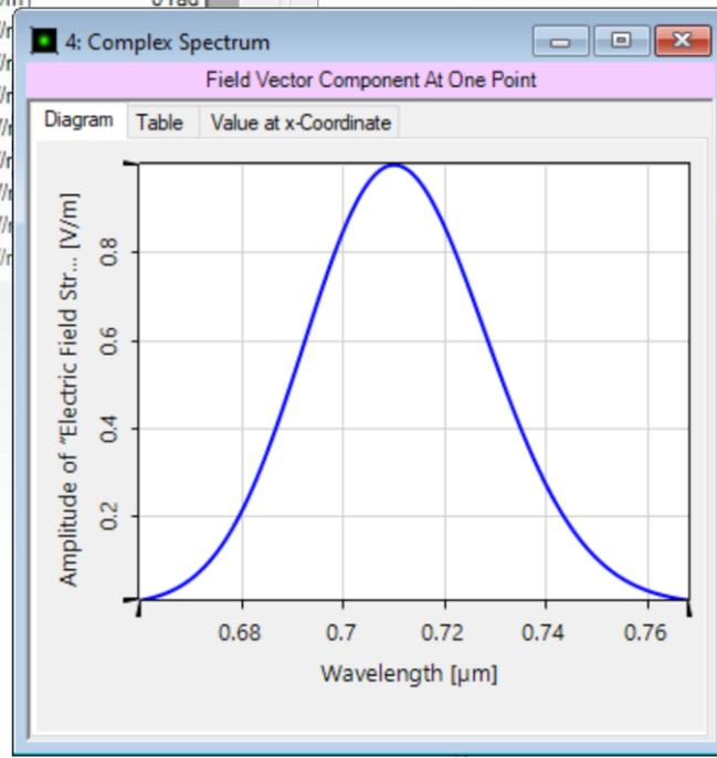
The source is modeled by applying a gaussian spectrum onto a two-dimensional gaussian distribution in space.
