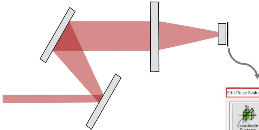
The detector automatically calculates the electromagnetic field in wavelength and time domain at a predefined point, line, or cube. It can also evaluate additional information like the optical path length and residual phase.
