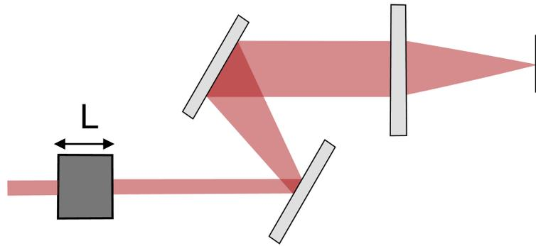
The grating pair introduces a chirp onto the field. If it is not compensated it will widen the pulse in time and therefore overlay the tilt.
