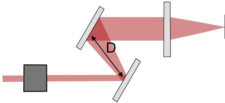
A higher distance between the gratings leads to a wider spectral separation which increases the tilt of the pulse front in the focus!
