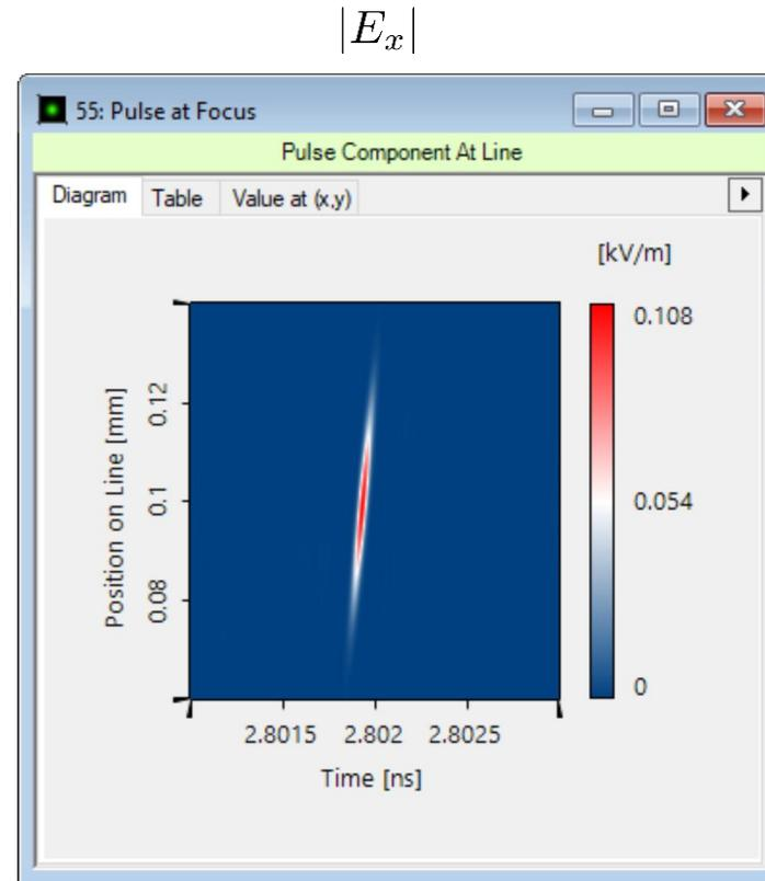
When the chirp generated by the system is functionally removed, the pulse in the focus shows a clear tilt. The angle of this tilt is depended on the focal length of the lens and the parameters of the stretcher.
