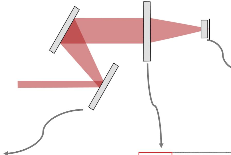
The chirp generated by the components of the system generally broadens the pulse. This effect can be negated by multiplying the negative residual phase onto the field.
