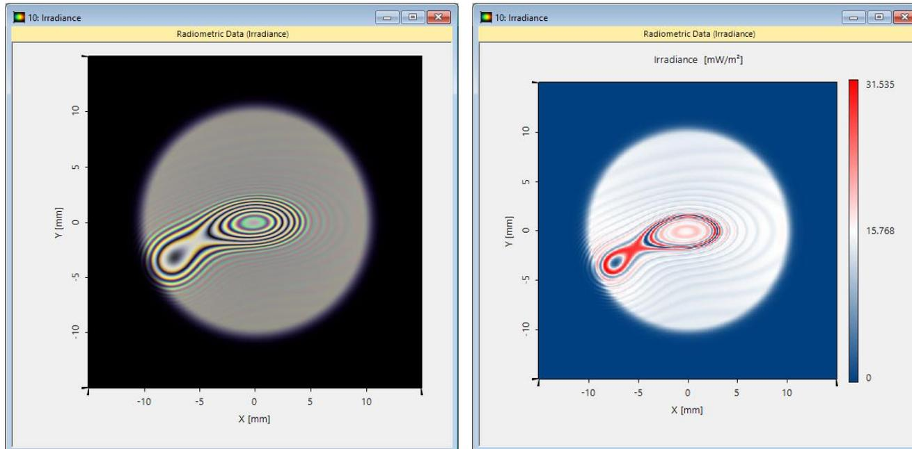
Full flexibility in detector modeling of different physical values, including irradiance, which can be given out in a predefined color-scheme or in the *Real-Color View*, which simulates how the human eye would see the result.
