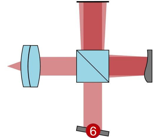
In this use case we investigate the effects of the specimen. Hence, for the other mirror of the interferometer we employ an idealized beam splitter model since we do not want to investigate e.g. the Fresnel losses that appear there. Therefore, a **Functional Approach** is sufficient.
