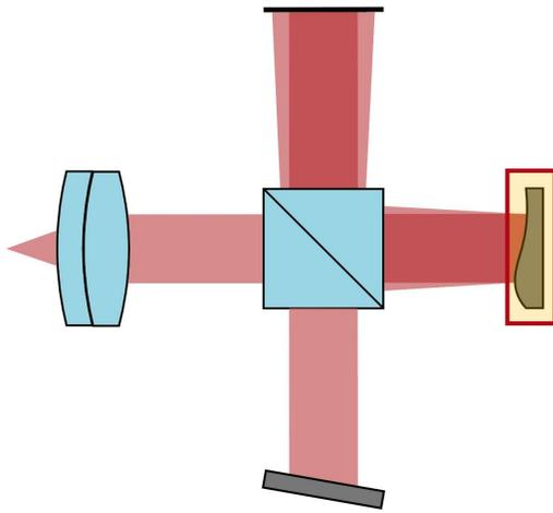
To incorporate the specimen with a custom height profile, VirtualLab offers the *Sampled Surface*, which can import arbitrary structures as long as their height information is given in a *Data Array*.
