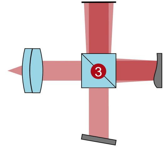
The choice of an appropriate modeling technique for a beam splitter heavily depends on which kind of beam splitter is used. In this use case we employ an idealized beam splitter model since we in principle have no interest in investigating e.g. the Fresnel losses that appear in the beam splitter, hence a **Functional Approach** is sufficient.
