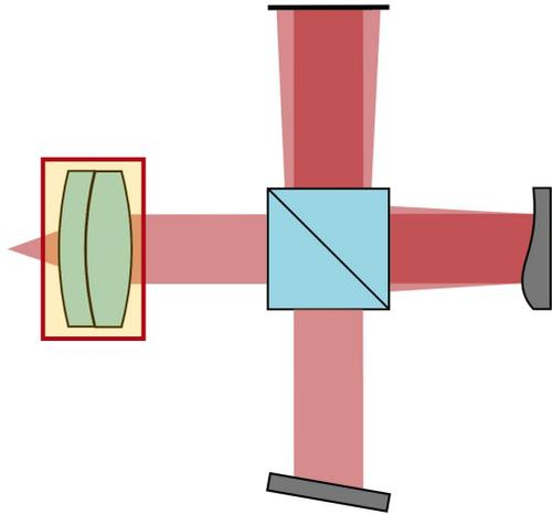
The *Lens System Component* allows the user to easily define a component consisting of an alternating sequence of smooth surfaces and homogeneous, isotropic media. For both interfaces and materials, you can choose ready-made entries from the built-in catalogs or customize your own for maximum flexibility.
