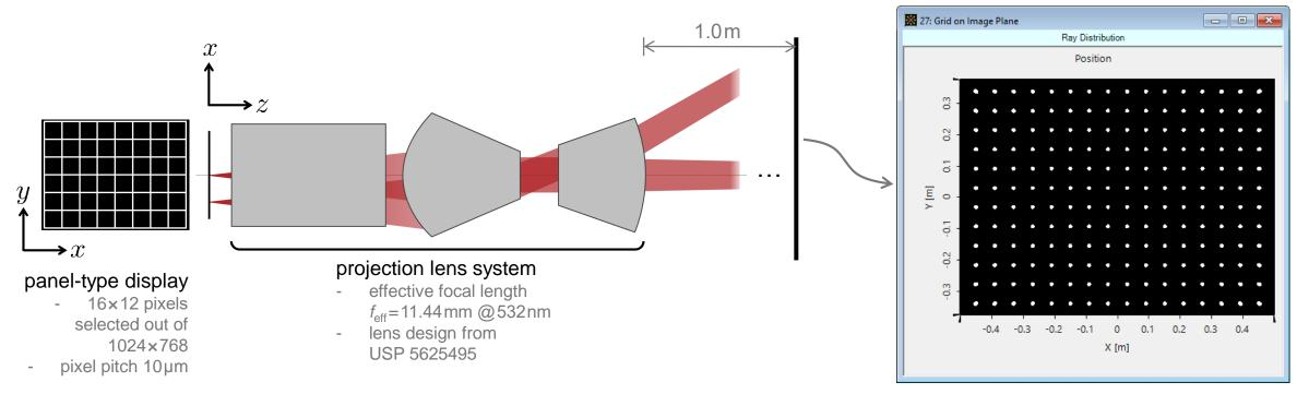
A well-designed projection lens system delivers an almost equidistant grid on image plane, with distortion under control.
