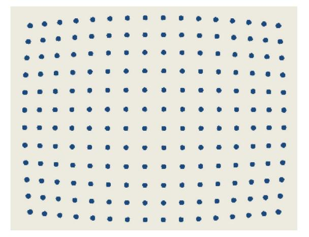
The modern display devices, e.g., liquid crystal display (LCD), are often used as the source for an imaging or projection system. Such display devices can be modeled conveniently by using the paneltype source in VirtualLab. As an example, an image projection lens is selected and analyzed with a panel-type source. The performance of the system is evaluated by both observing the spot grid in the image plane, and evaluating the angular/direction behavior.
