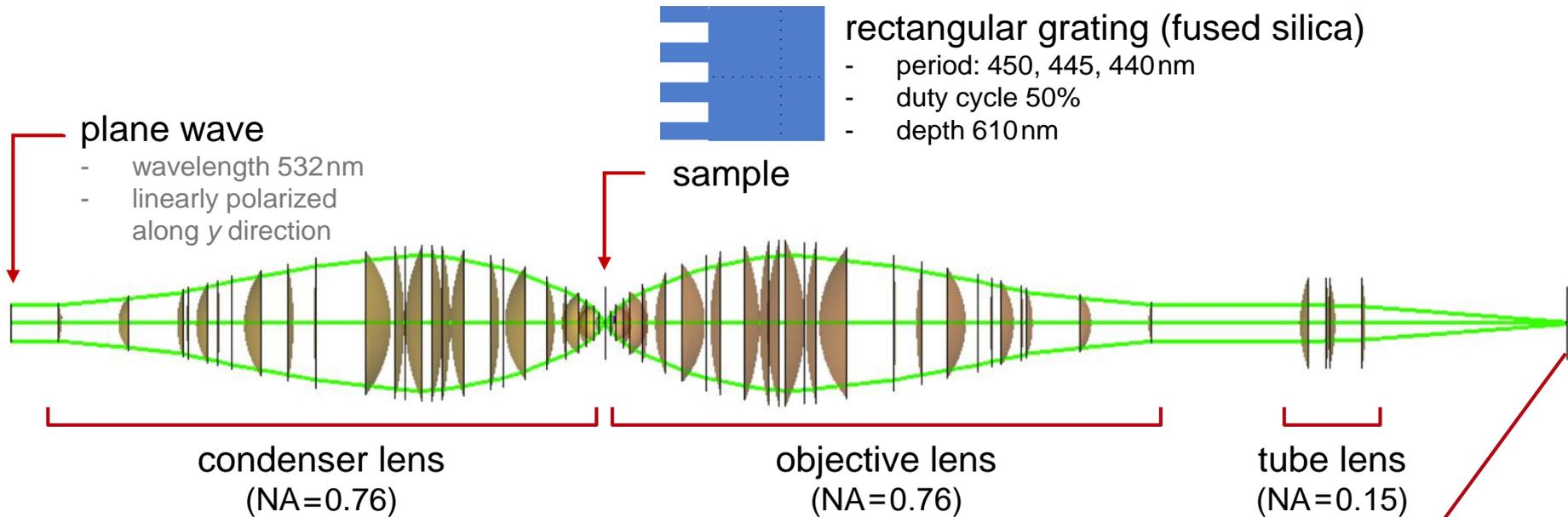
How to calculate the image of the sub-wavelength grating, taking the grating diffraction and vectorial effect in high-NA system into account?
