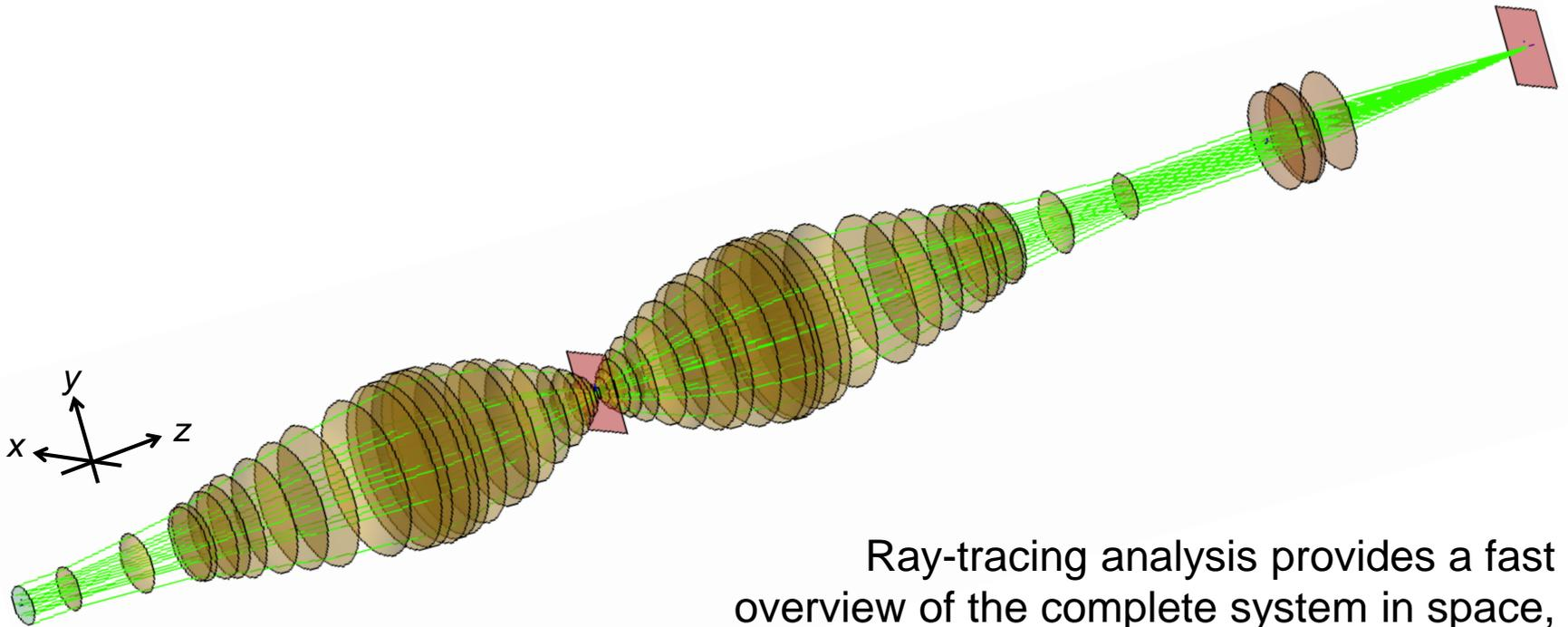
Ray-tracing analysis provides a fast overview of the complete system in space, including multiple diffraction orders.
