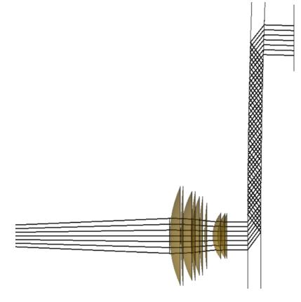
In a near-to-eye display system, the image generation unit, the collimation optics, the waveguide and the in- and outcoupling gratings, form a complex folded imaging system. To evaluate the image quality of such systems, it is important to include the influence from the waveguide structure. In this example, a folded imaging system, with either a planar waveguide or a curved waveguide, is modeled, and the PSF and MTF on image plane are calculated.
