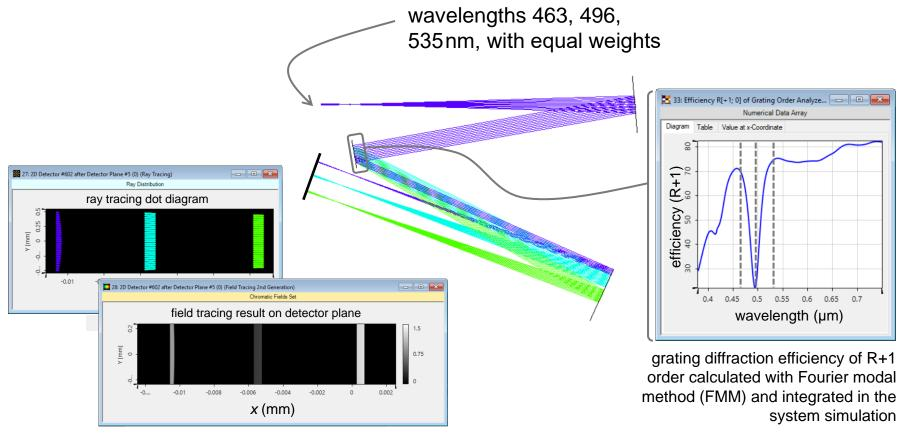
Simulation of full system including rigorous grating simulation takes only 3 seconds.
