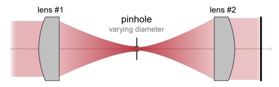
Spatial filter in the Fourier plane helps reduce the higher-frequency noise, therefore leads to better output beam profiles.
