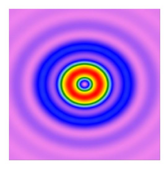
The emission light of a fluorescent molecule and the scattered light of a nanosphere are well modeled by dipole sources. Therefore, a dipole source is a good model for a point source which considers the vectorial effects in practice. Analysis of the PSF of such point source is important. The dipole source is built in VirtualLab Fusion. By connecting with a complex high-numerical-aperture microscopy system, the PSF is directly calculated in VirtualLab Fusion.
