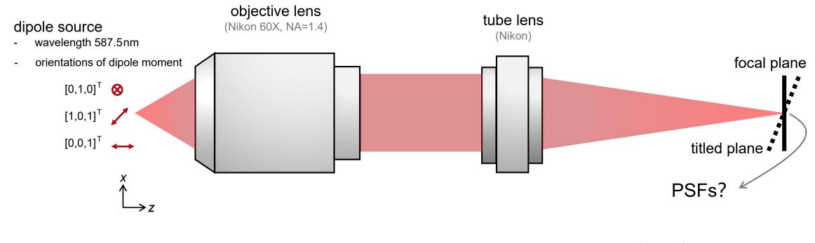
What are the PSFs of a dipole source with different orientations? And what are these PSFs on the tilted plane?
