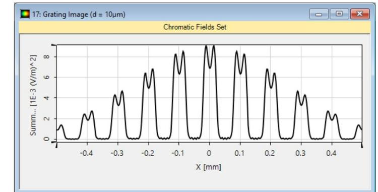
Due to the loss of high spatial frequencies, the image of the grating with smallest period clearly deviates from the object.
