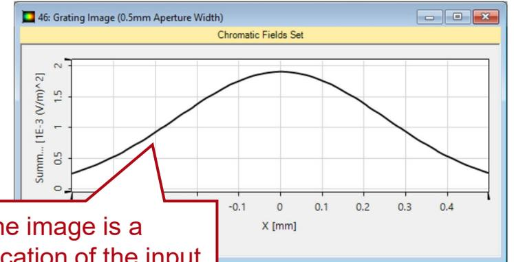
The image is a magnification of the input Gaussian beam.
