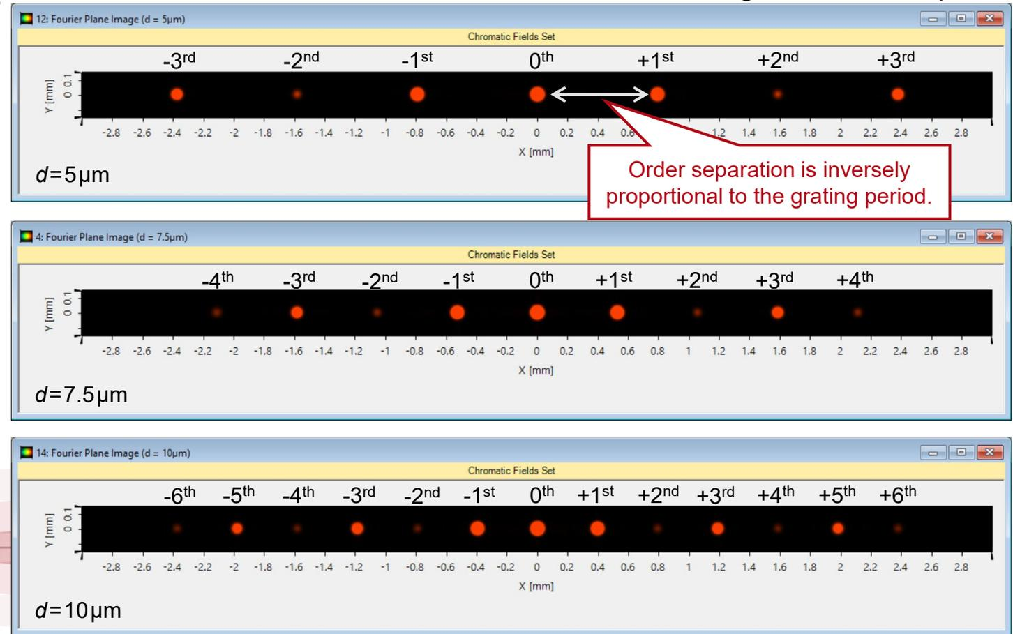
Grating efficiencies – corresponding to the spot brightness – are calculated by Fourier modal method (FMM, also known as RCWA).
