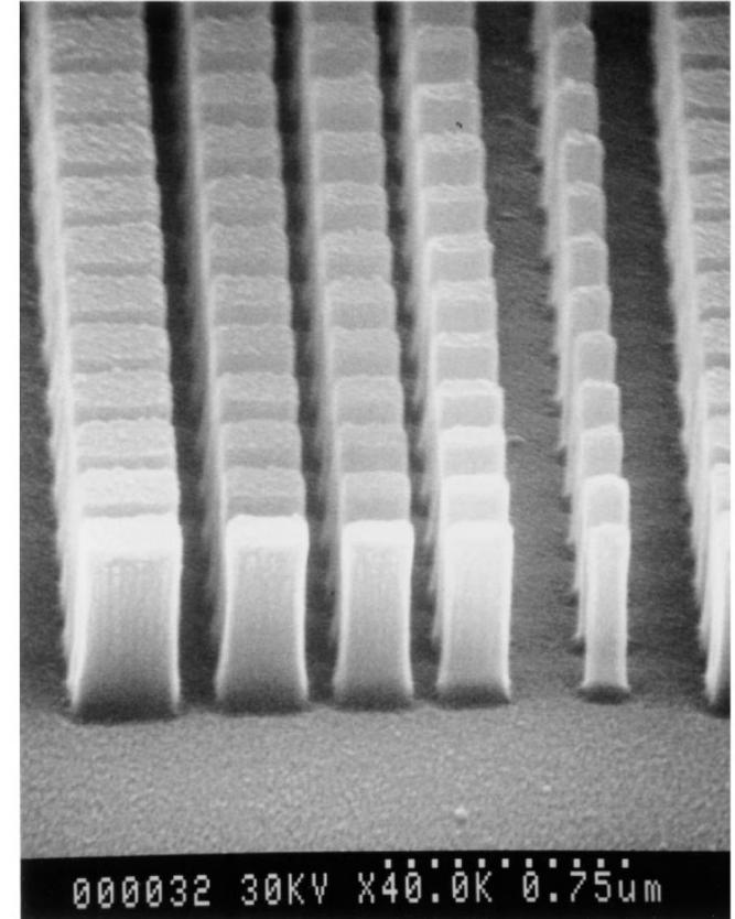
Fig. 2. Scanning-electron micrograph of the blazed binary subwavelength grating. The horizontal period (along the  $x$  axis) is  $1.9 \mu\text{m}$ , and the period in the perpendicular direction ( $y$  axis) is equal to the sampling period (380 nm). The maximum pillar aspect ratio is 4.6.
