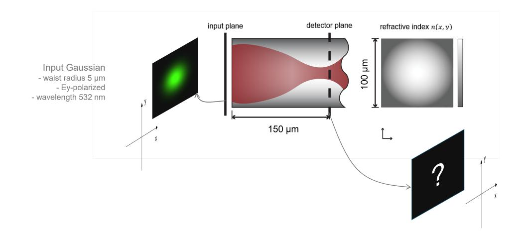
calculate the result fields by Fourier modal method and Runge-Kutta based kdomain algorithm.
