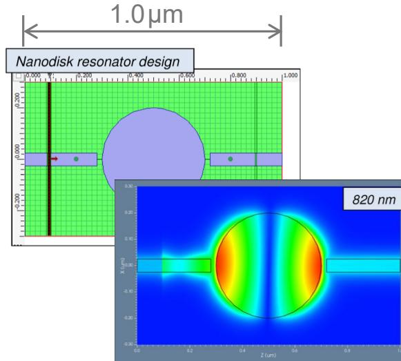
Plasmonic waveguide filters with
