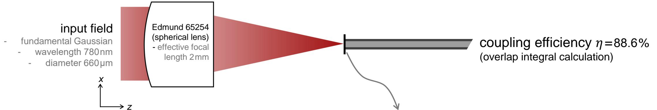
How to modeling such an optical system for fiber coupling?
