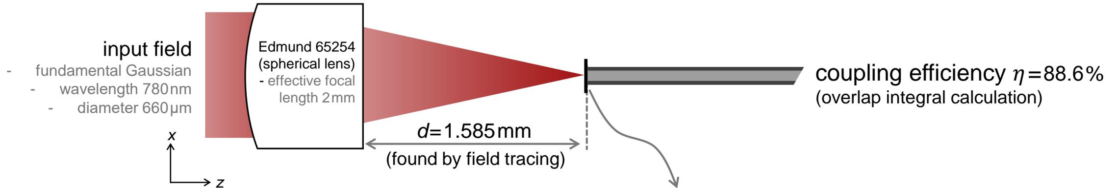
The calculation of the focal spot and the evaluation of the coupling efficiency takes only 2 seconds!
