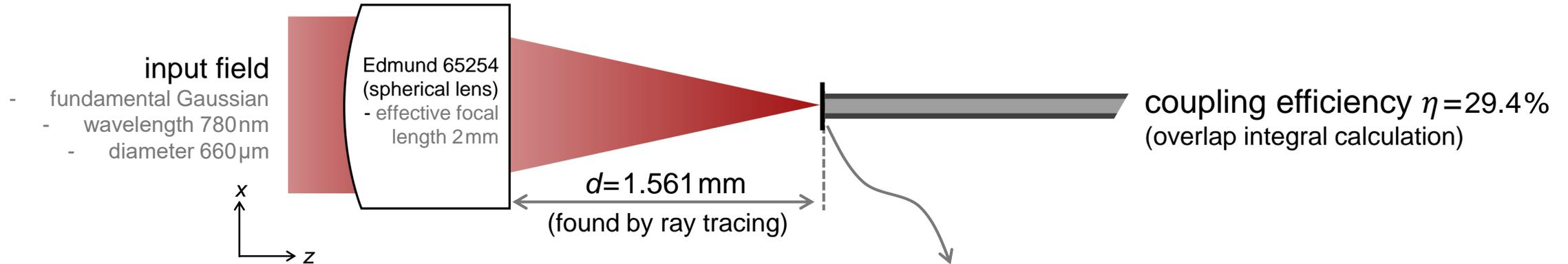
Field tracing in VirtualLab provide access to the full field information at any desired plane in the system.
