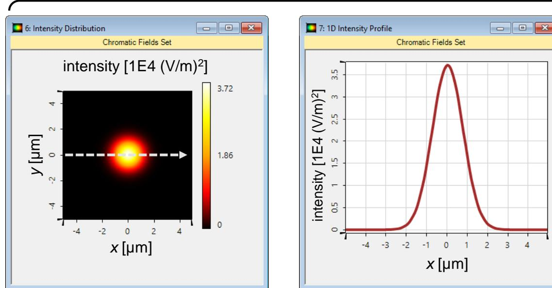
Field tracing simulation of the fiber coupling system takes only 2 seconds.
