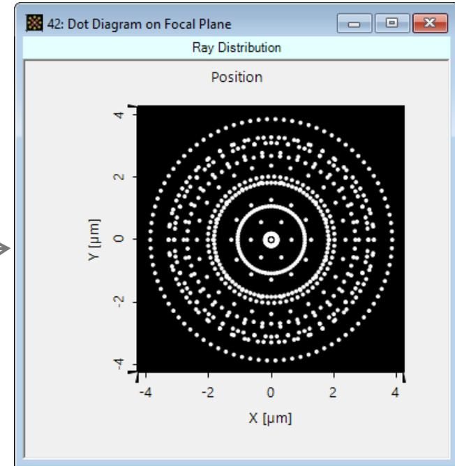
The beam diameter (RMS) evaluated with ray tracing is  $5.11 \mu\text{m}$ .
