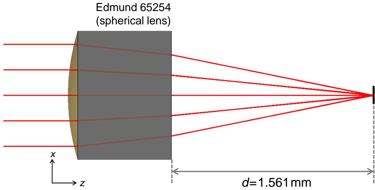
Focal distance for the spherical lens is found first by using ray tracing in VirtualLab.
