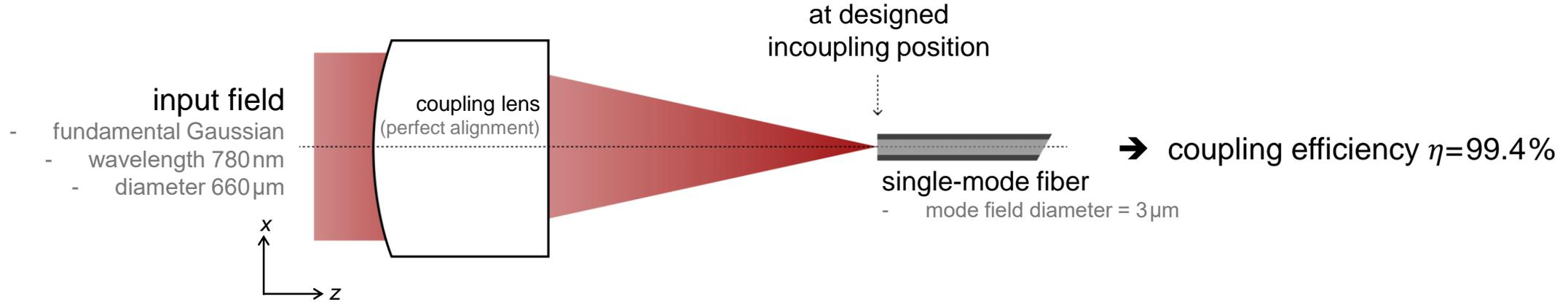
How does the coupling efficiency change with respect to alignment tolerance factors?
