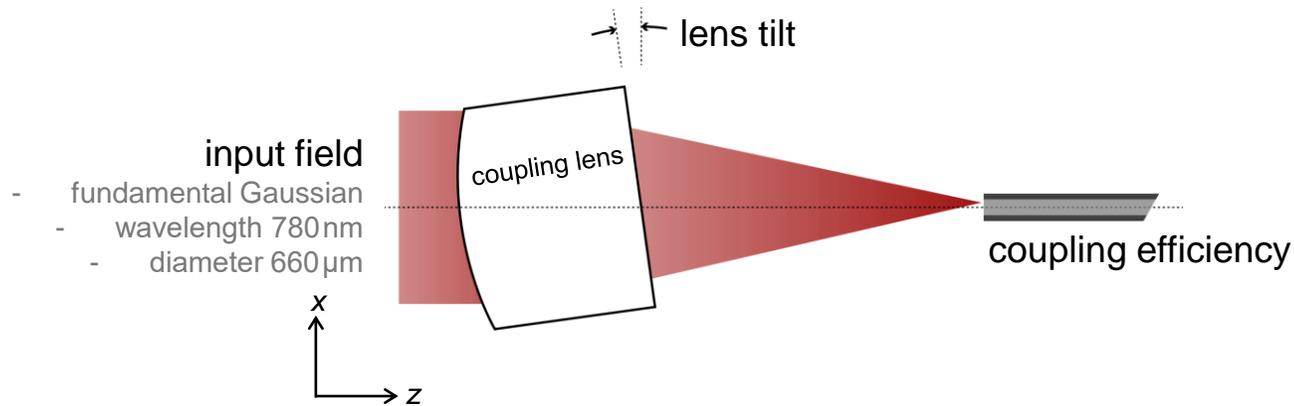
Physical-optics analysis of the coupling efficiency with respect to lens tilt, over 200 angles, takes only 50 seconds.
