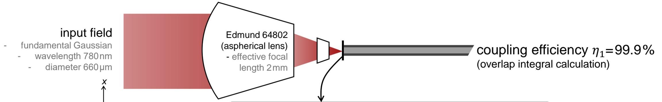
Aspherical lens controls the aberrations well and that guarantees a focal spot in smaller size, and with Gaussian profile that fits to the fiber.
