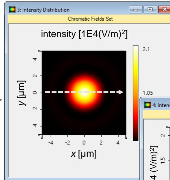
The coupling efficiency obtained from the initial spherical lens is not optimal, due to mismatch to the mode inside the single-mode fiber.
