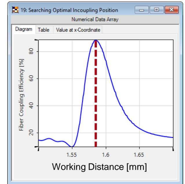
The optimal working distance found by field tracing is 1.585 mm.
