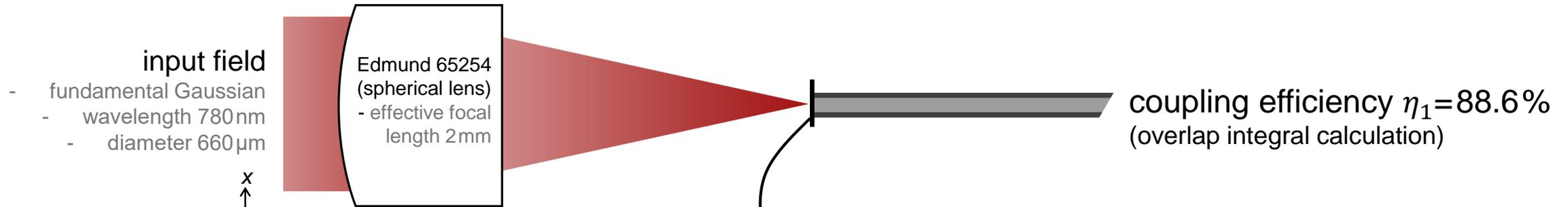
Due to aberrations from the spherical lens, the focal spot at the end of the fiber deviates from a Gaussian mode, and therefore it leads to poor coupling efficiency.
