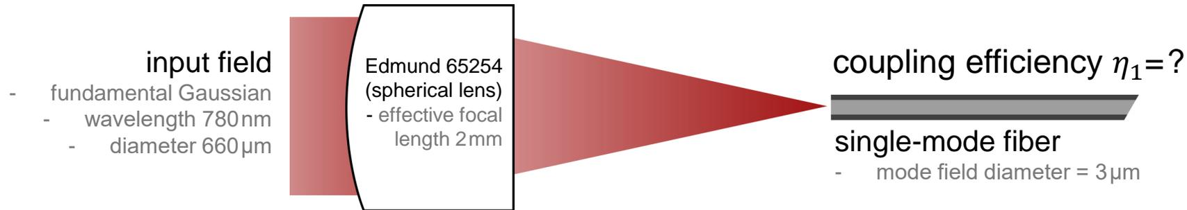
When two lenses with the same effective focal length are available for fiber coupling task, how to evaluate their performance in terms of coupling efficiency?
