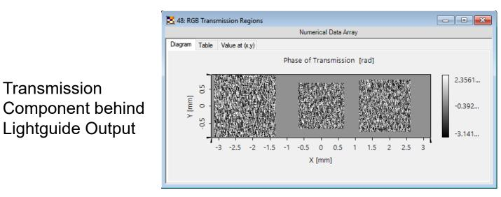
The designed transmissions are combined to a single transmission, which is located at the output of the Lightguide component.
