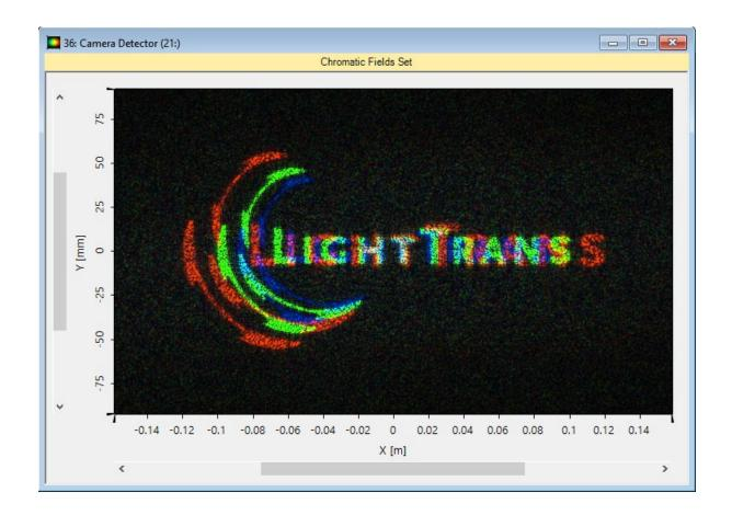
The transmissions designed for 532nm is analyzed by propagating RGB with far field operator (as comparison for the final result).
