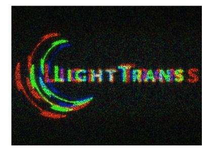
In this demo we show how to design a diffuser for distinct target pattern for each of the RGB wavelengths. Furthermore, we will generate a Lightguide setup for guiding and separated outcoupling of the RGB modes. In the last step, we apply the diffuser transmission functions to the outcoupled modes and propagating them into the far field to generate white light pattern.
