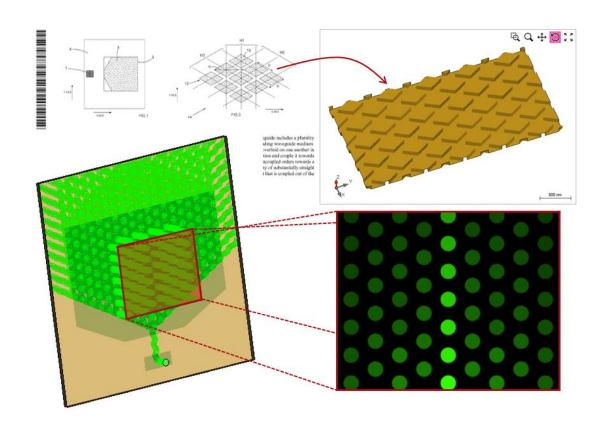
Most innovative AR & MR devices nowadays are based on lightguide or waveguide systems in combination with microstructures for in- and outcouple of the light. VirtualLab Fusion is capable of detailed modeling of such devices by applying our unique physical optics approach, including all effects (e.g. coherence, polarization and diffraction). We demonstrate this capability by modeling a device mentioned in patent WO2018/178626, consisting of complex 1D and 2D-perodic grating structures.
