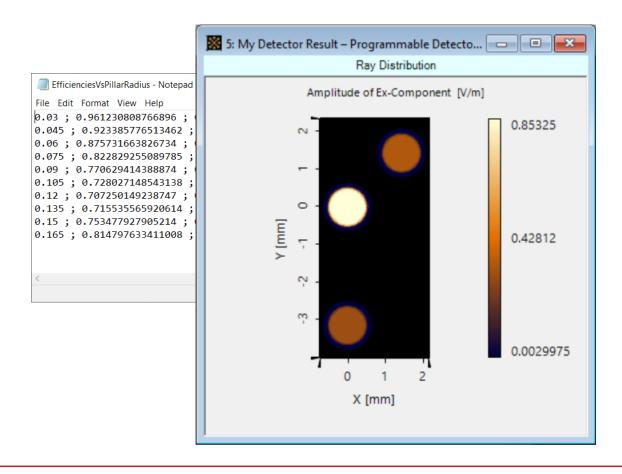
This Demo shows how to use precalculated efficiency to define a grating in VirtualLab Fusion.
