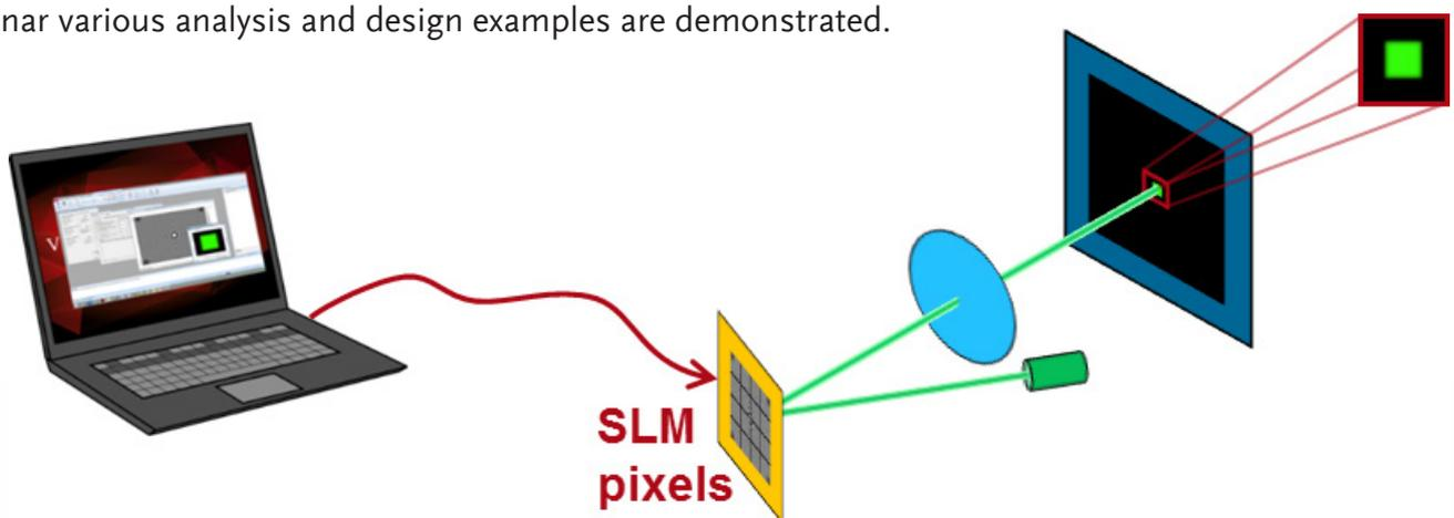
*Design and simulation of required phase values for actuating a spatial light modulator (SLM) module in order to generate a top-hat.*
