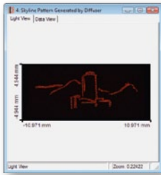
Diffuse light pattern generated by a diffractive diffuser.
