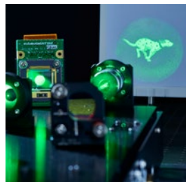
Light shaping by a spatial light modulator (SLM), diffraction efficiency > 90°
