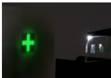
Green LED light shaped into a cross pattern by a grating cells array
