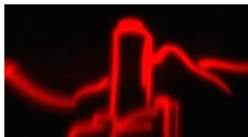
Skyline of Jena generated by a diffractive diffuser illuminated by a red LED
