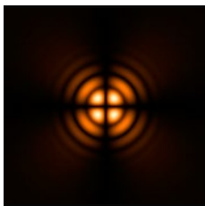
Y-component of the electric field in the focal region of a high-NA lens
