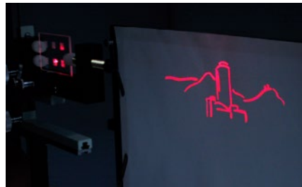
High-NA diffractive diffuser, field-of-view: 120 degrees
